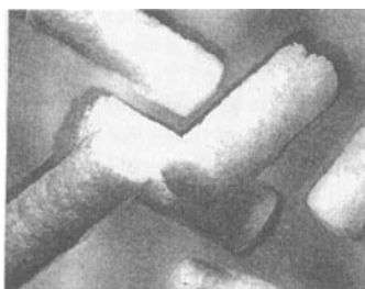
Fig. 4. Loose fillers made of Mater-Bi of class V (starch content higher than 85 %)
